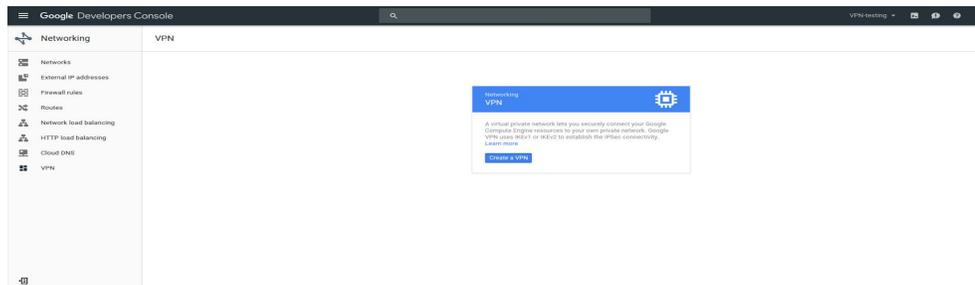
All parameters needed to create a new VPN connection are entered on this page. Provide a **Name** and **Description** for the VPN instance. The VPN instance requires a **public IP address**. An existing address can be selected if available, or a **New static IP address** can be assigned:
